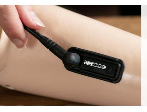
The S-Charge System is a user friendly, powerful internal battery system, with an OLED display and a magnetic charger which can all be installed into a prosthesis. This allows the user to easily activate, deactivate, and charge their prosthesis while confidently monitoring the power status during the day.
