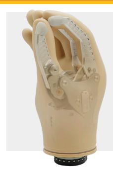
The Myo Kinisi is a myoelectrically controlled terminal device engineered to provide optimal control, responding intuitively to the strength and speed of the user's muscle contractions. This prosthetic hand is designed to be tailored by the prosthetist to the individual's needs, with multiple wrist, size, and hand mode options for the patient's comfort and usability.
