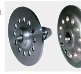
Adaptor Plates have 2 variations; one with the holes to provide free rotation with locking in any 1 of the 12 positions, and one with this feature removed to allow free rotation without locking.
